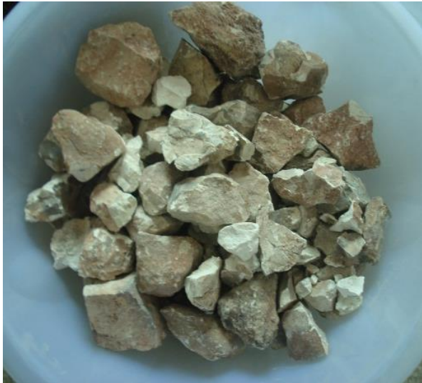
Figure 4: Quick (white) Lime produced after burning of limestone
