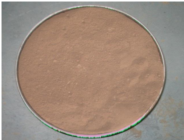
Figure 2: Fine ground, fully calcined kankar lime.
