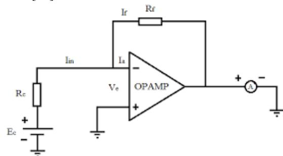
Figure 10. Zero Resistance Ammetry Circuit Diagram [24].
