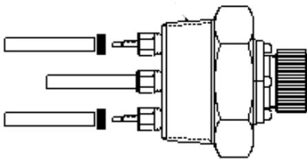
Figure 8. Linear Polarization Resistance Probe[15]
