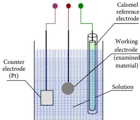
Figure 7. A Sample Three Electrode Cell with Platinum (Pt) Counter Electrode and Calomel Reference Electrode [24].
