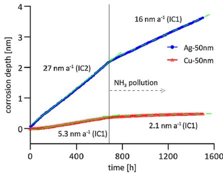
Figure 3. Corrosion depth VS. time for copper and silver[12].
