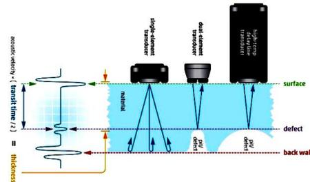
Figure 1 Wall Thickness being measured using ultrasonic transducers [37].
