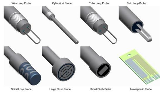
Figure 5. Types of electrical resistance probes[15]
