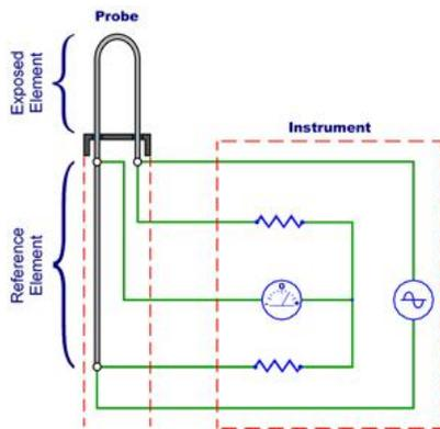
Figure 4. Electrical Resistance Probe [15]
