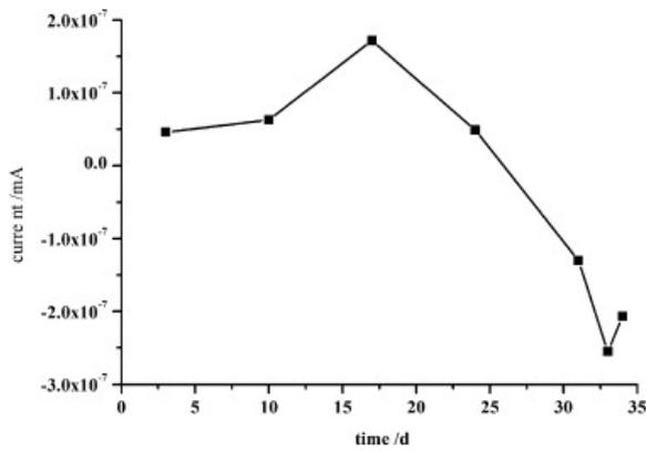
Figure 11. ZRA measurement of copper and iron electrodes [31].
