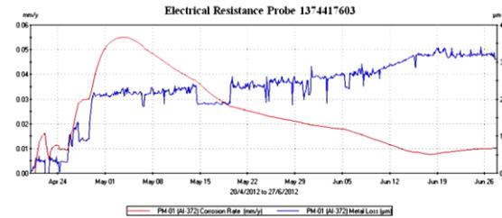
Figure 6. Corrosion rate and loss of material thickness represented against exposure time to corrosive media [18].
