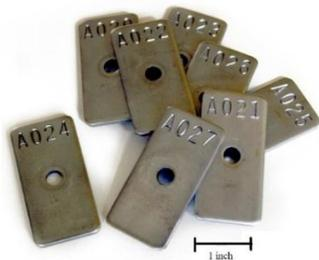
Figure 1. GMW14872 standard mass loss coupons According to GM9540P, the coupons are eligible to be removed after 8 cycles[13].
