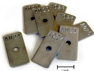
Figure 1. GMW14872 standard mass loss coupons According to GM9540P, the coupons are eligible to be removed after 8 cycles[13].
