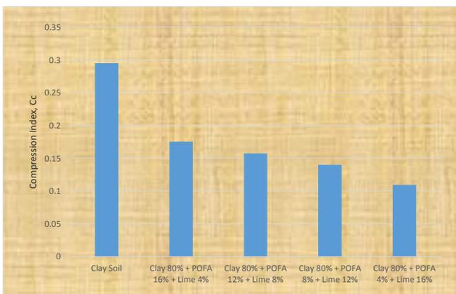
**Figure (3): Compression Index (Cc) for Clay Soil and Stabilized Sample**
