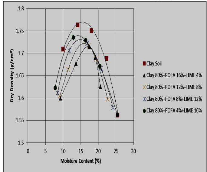
**Figure (2): Compaction Curve Graph for Clay Soil and Stabilized Sample**
