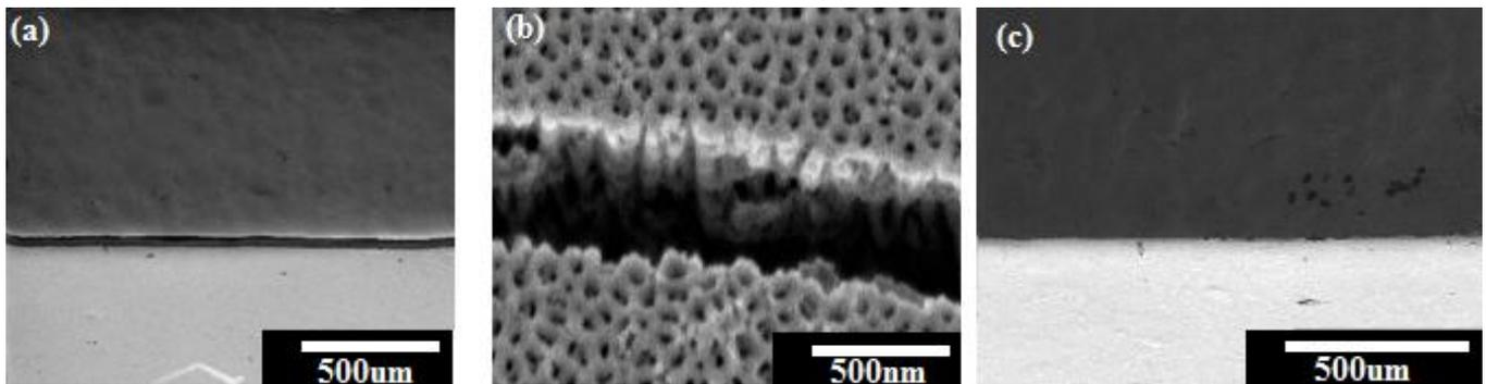
**Fig (1) FE-SEM images of solid alumina edges: (a) Formation of crack at 3D sharp angle (b) magnified image showing the crack (c) 3D crack free dull angle edge having high radius of curvature.**
