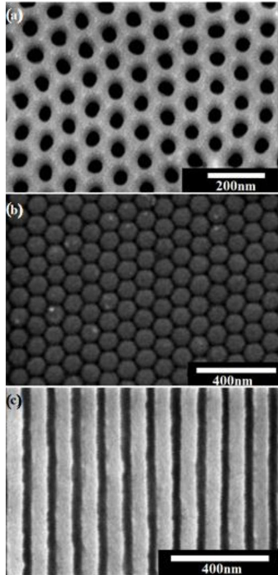
**Fig (4) SEM images of self-organized AAO structures (a) uniform hexagonal pore planar surface structure, Fig. 4 (b) shows barrier layer (c) nanochannel cross section image**
