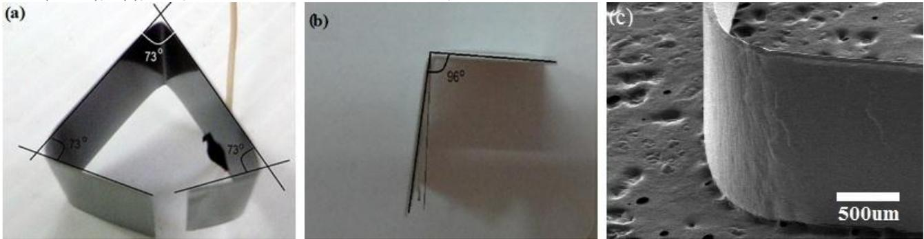
**Fig (3) Optical and SEM images of the AAO grown structures (a) triangular structures which clearly show the expansion of angle from 60° to 73° ultimately released mechanical stress, avoiding cracks as shown in Frg.4 (b) in the Fig.4 (c) uniform diameter nanochannel perpendicular to the surface.**
