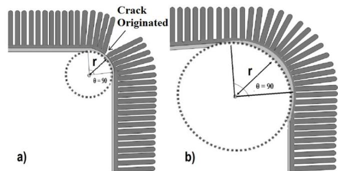
**Fig (2) Schematic of the anodization at bends, (a) crack formation at sharp angle having very small radius, (b) no any crack appeared in the structure due to large value of radius to angle ratio**
