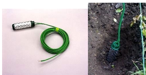
Fig 2: ES1100 Watermark Sensor (source memsic.com)
