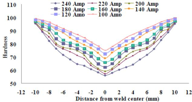
**Figure 5: Microhardness profile effected by AC (100 – 240A) [28].**
