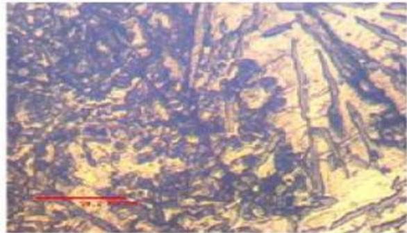
Figure 4a: Microstructure of HAZ for 80A [26].
