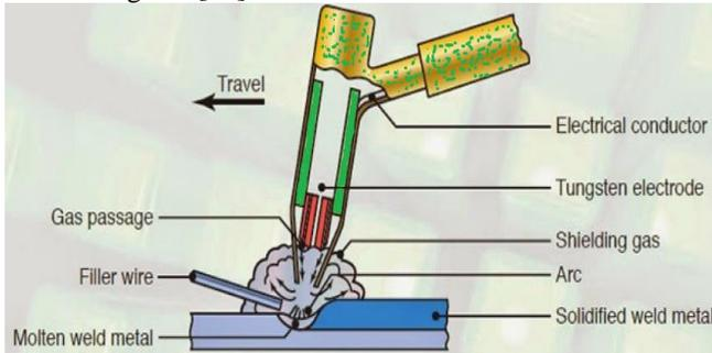
Figure 1: Gas Tungsten-arc Welding Process [16].
