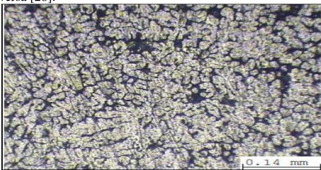
**Figure 8: microstructure of weld metal at 140A [28].**
