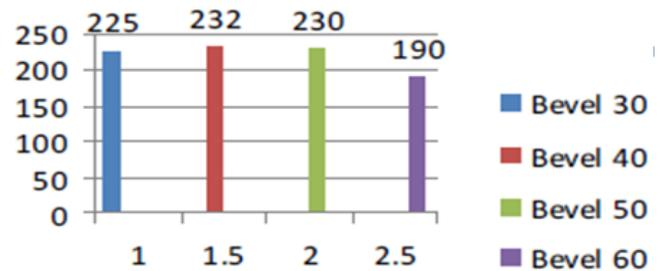
**Figure 7: Tensile graph of different bevel angle at 0.6 cm / sec welding speed [22].**
