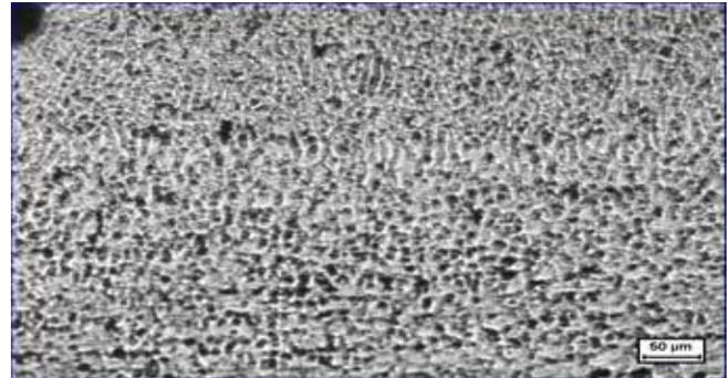
**Figure 9a: Heat Affected zone microstructure using argon at 14 L/min flow rate [25].**
