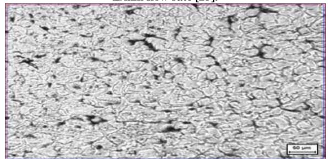
**Figure 9b: Heat Affected Zone microstructure using Helium at 6 L/min flow rate [25].**
