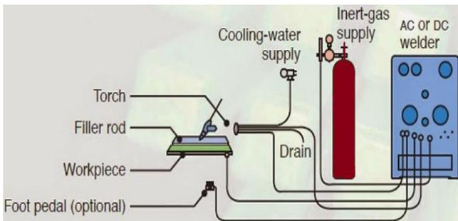
Figure 2: Schematic diagram of Operation and Equipment (TIG) welding [16].
