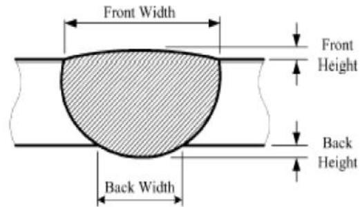
Figure 3: Geometry of weld bead [20].
