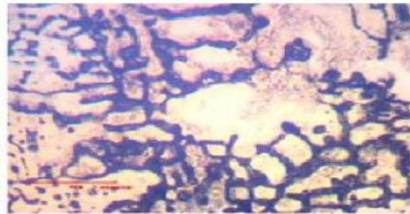
Figure 4b: Microstructure of HAZ for 75A [26].
