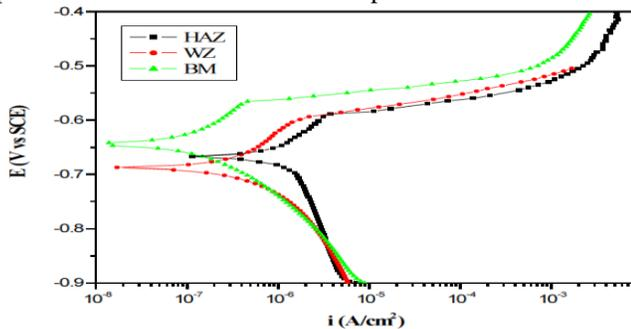
**Figure 11: Polarization curves (Anodic and cathodic) for Aluminum Alloy 2219-T87 in seawater [33].**
