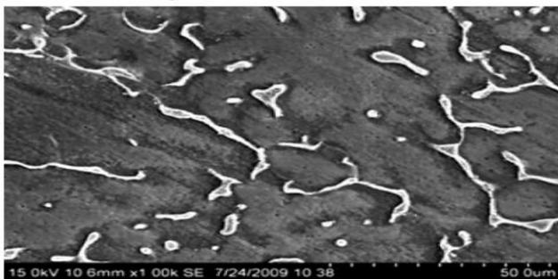
**Figure 12: SEM image of Heat Affected Zone [33].**
