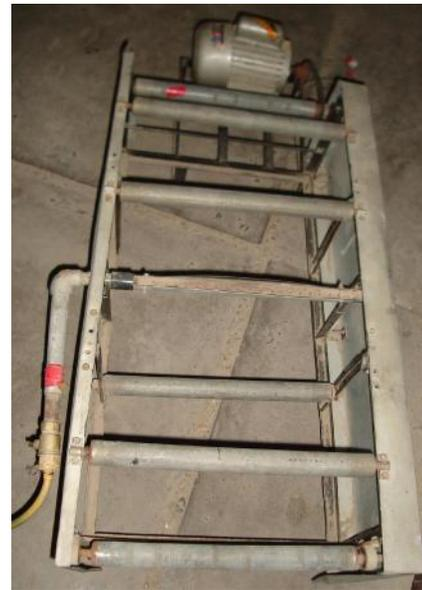
Fig. 4: The Laboratory Singeing Machine (Top View)
