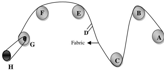
A = Let-off roller, B, C, E and F = Tension rollers, D = Burner, G = Take-up roller, and H = Motor.
