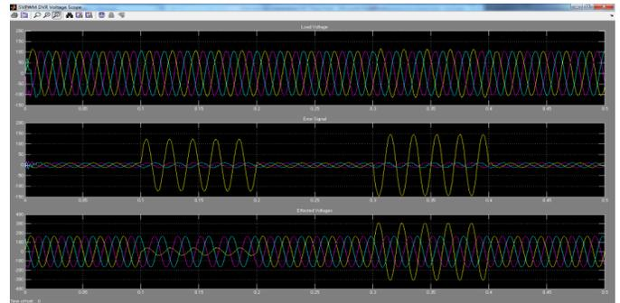
**Figure-7 Single phase voltage Compensation with DVR**
