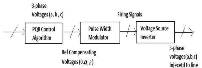
**Figure-2 Control flow of DVR controller**
