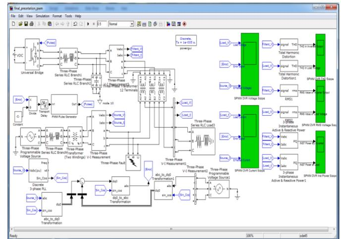
**Figure 4 Matlab/Simulink based System Model.**
