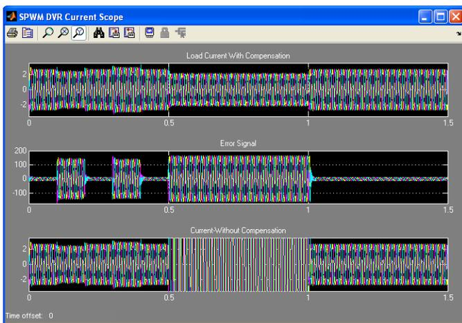
**Figure-6 Load Current Compensation with DVR**
