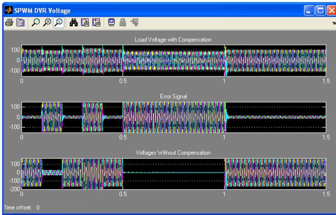
**Figure-5 Three phase voltage compensation with DVR**
