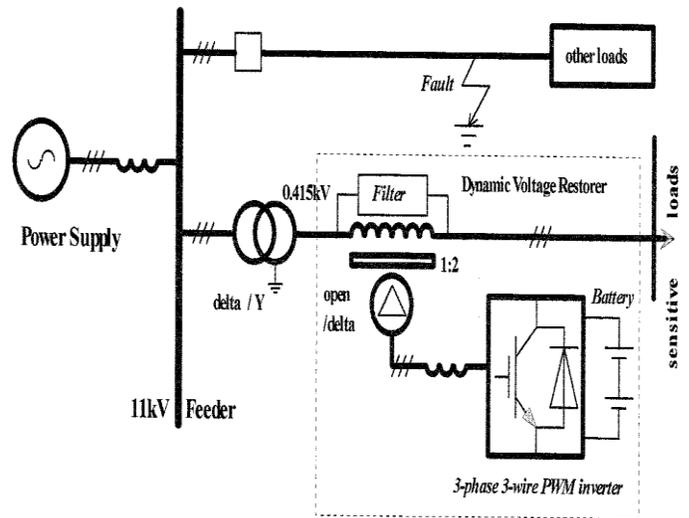
**Figure-1 Schematic DVR main circuit**
