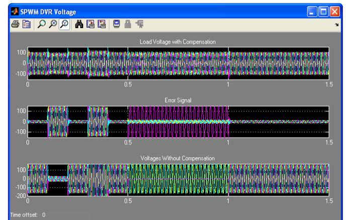
**Figure-4 Single phase voltage Compensation with DVR**
