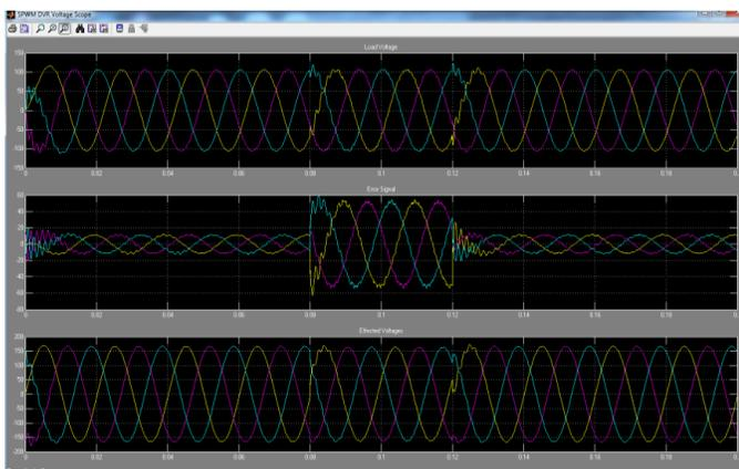
**Figure-7 Phase disturbance in Supply Voltage and compensation for sag / swell**
