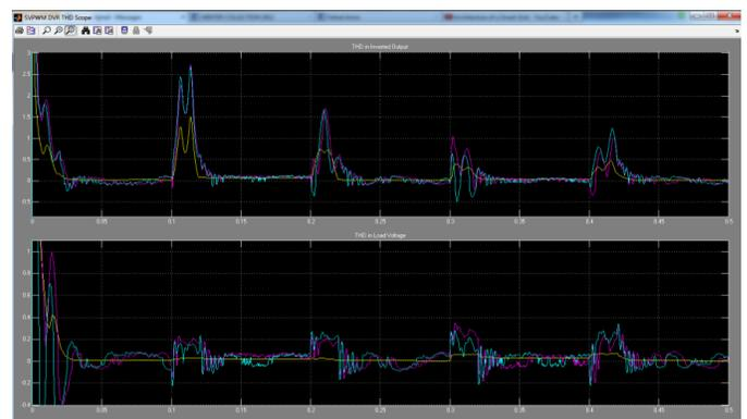
**Figure-9 Harmonic distortion during disturbance.**
