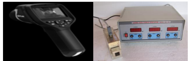
Figure 7: Flir E60 Infrared Thermal Camera (left) and Force dynamometer (right)
