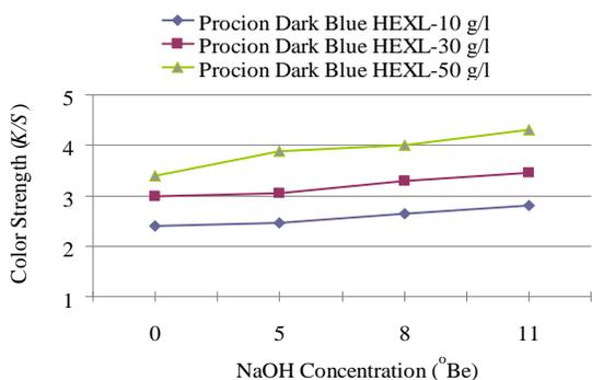
Fig. 4: Colour Strength of Lyocell Fabric Dyed – Pad-Dry-Cure Method (0-11°Be NaOH)
