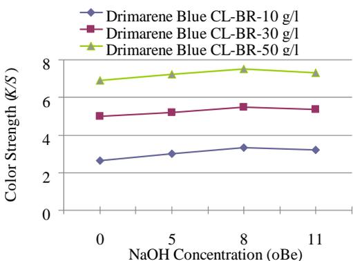
Fig. 5: Colour Strength of Lyocell Fabric Dyed –
