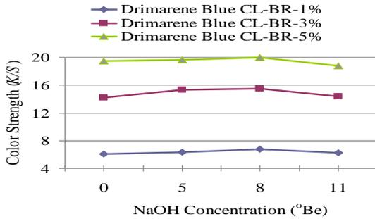
Fig. 3: Colour Strength of Lyocell Fabric Dyed – Exhaust Method (0-11°Be NaOH)
