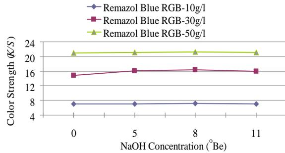
Fig. 6: Colour Strength of Lyocell Fabric Dyed by Pad-Batch Method (0-11°Be NaOH)
