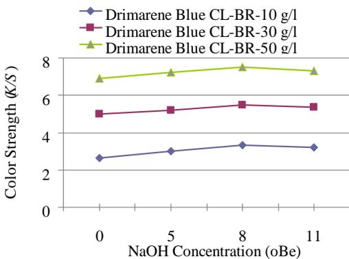
Fig. 5: Colour Strength of Lyocell Fabric Dyed – Pad-Dry-Cure Method (0-11°Be NaOH)
