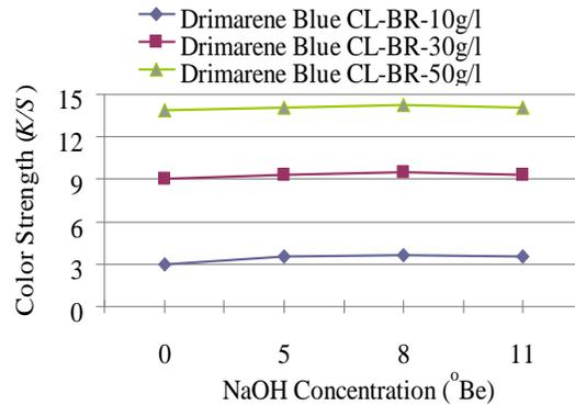
Fig. 7: Colour Strength of Lyocell Fabric Dyed by Pad-Batch Method (0-11°Be NaOH)
