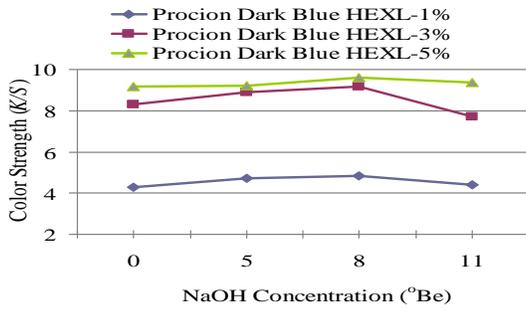
Fig. 2: Colour Strength of Lyocell Fabric Dyed – Exhaust Method (0-11°Be NaOH)
