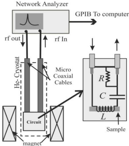
**Fig.3: The schematic diagram of the proposed setup for radio frequency transmission through the band pass circuit in dc field magnets and at liquid Helium temperatures.**
