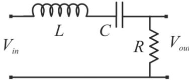
**Fig.1: The circuit diagram of a band pass filter circuit, where  $L$  is the inductance of the coil,  $C$  is the capacitance,  $R$  is the resistance,  $V_{in}$  and  $V_{out}$  are the amplitude of the input and the output of rf signals.**
