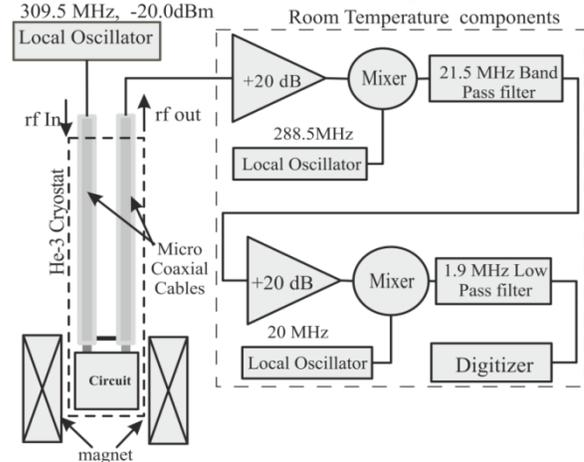
**Fig.4: The schematic diagram of the experimental setup for radio frequency signal transmission through the band pass circuit in pulsed magnet and at liquid He4 temperature.**
