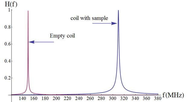
**Fig.2: The band pass circuit reponce function  $H(f)$  magnitude as a function of frequency for an empty coil and for loaded coil. The values in Eq.2 and Eq.4 were chosen as:  $R = 0.6\Omega$ ,  $C = 5.0\text{pF}$ ,  $= 1 \times 10^{-9}\Omega.m$ ,  $r_{coil} = 0.75\text{mm}$ ,  $r_s = 0.70\text{mm}$  and  $n = 20,000$  turns /m.**
