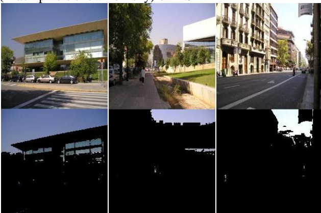
Figure 6: Result of Multilayer Perceptron classifier on DS1. First row shows original images, second row shows the result (Black pixels show non-sky) on DS1.
