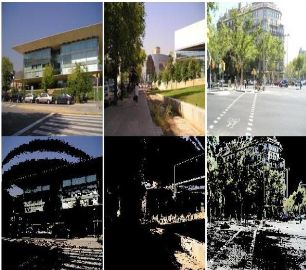
Figure 10: Result of applying the Radial Basis function classifier. First row shows original images, second row shows the result of the Radial Basis function (Black pixels show non-sky) on DS1
