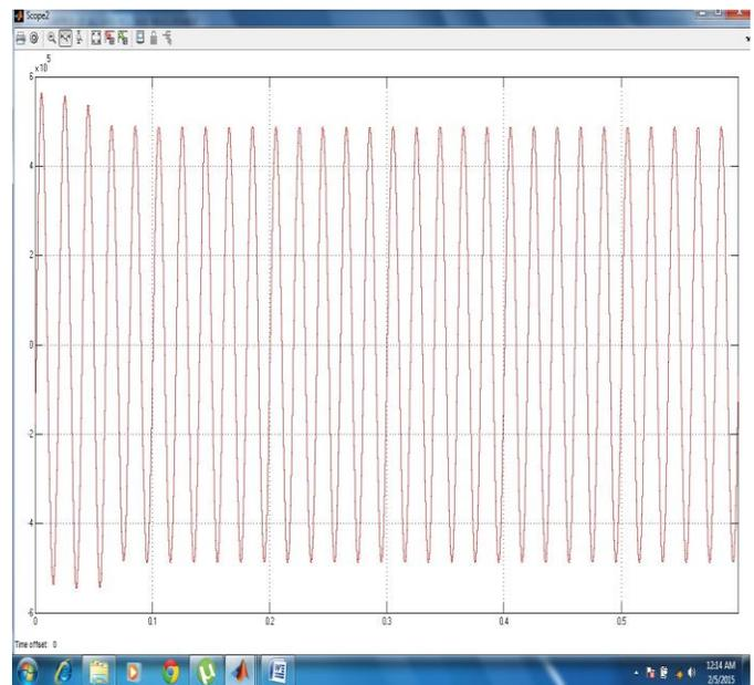
**Figure- 10 500KV Bus Bar Voltage during Phase-Ground fault.**
