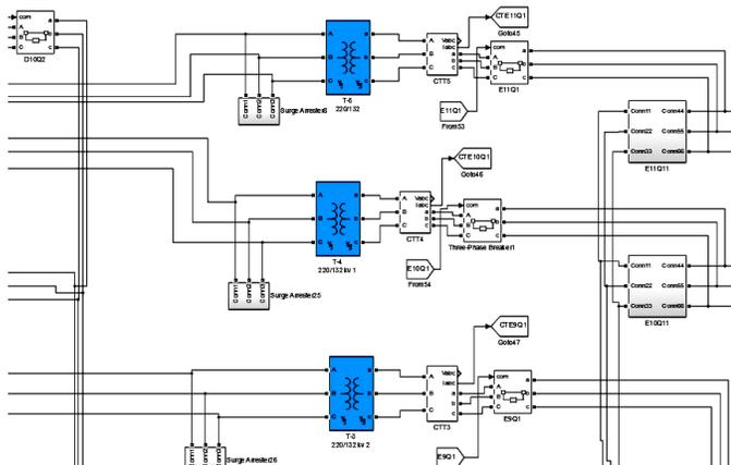
Figure 7: Matlab Model for 220/132 KV Transformers.
