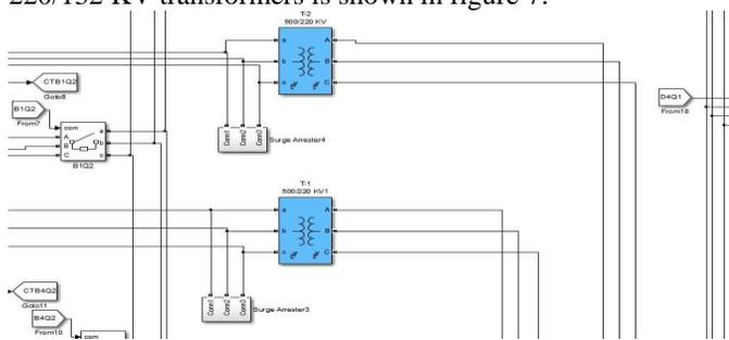
Figure 6: Matlab Model for 500/220 KV Transformers.
