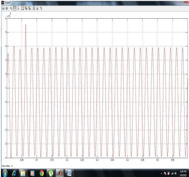
**Figure- 11 500KV Bus-Bar Voltage during Fault.**
