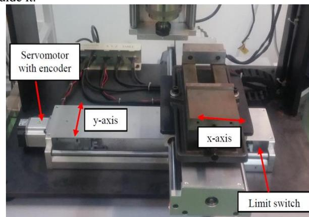
**Figure 1: Plant for the research: XY Table ball-screw drive system**
