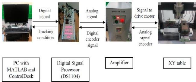
Figure 2: Schematic diagram of the experimental setup
