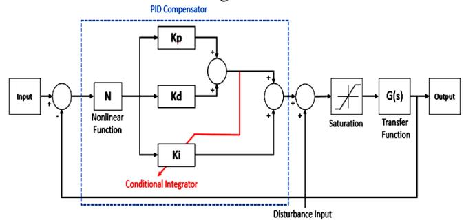
Figure 3: Control scheme of PID + iCON controller
