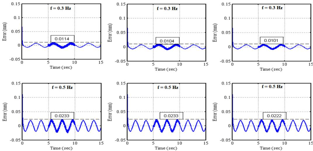
Figure 6: Result of maximum tracking error of PID + iCON Controller at  $f = 0.3$  Hz and  $f = 0.5$  Hz
