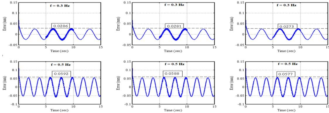
Figure 5: Result of maximum tracking error of PID Controller at  $f = 0.3$  Hz and  $f = 0.5$  Hz
