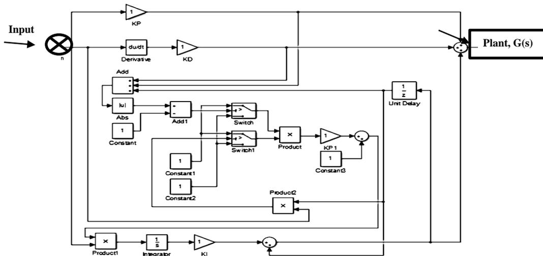
Figure 4: Method on how to integrate PID with conditional integrator
