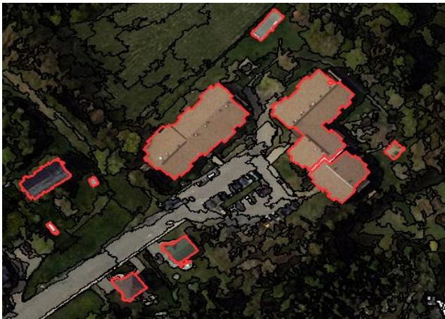
Figure 5. Segmentation Example of aerial image using object based methods [32].
