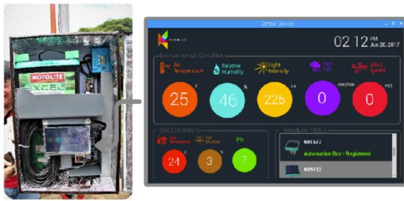
Figure 5. Central Device with the Sensors and LCD screen along with the readings from the sensors.
