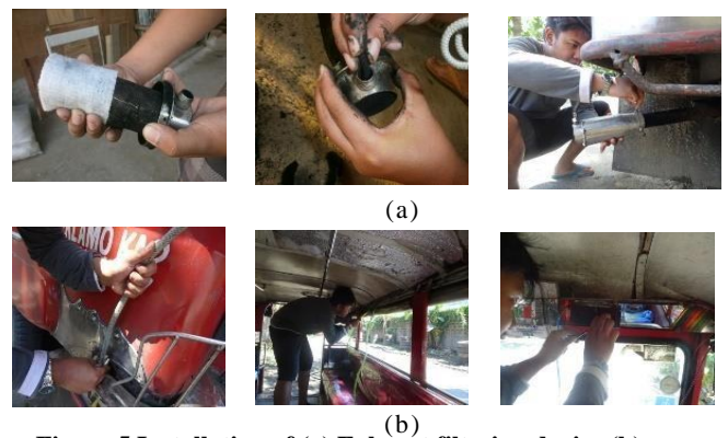
Figure 5 Installation of (a) Exhaust filtering device (b) Monitoring Device
