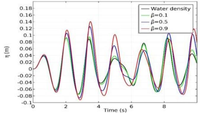
**Figure 5. Time histories of free surface profiles for various beta-value (Almost-homogeneous liquid), at position (x = L, y = W / 2) with  $\omega=4 \text{ rad/s}$**
