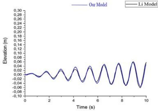
**Figure 4. Comparisons of free surface elevation at the left wall of the container for  $X_0 = 0.0004 \text{ m}$  and  $\omega = 5.0502 \text{ rad/s}$ , between the present numerical model (black line) and the numerical results by Lu et al. (red line).**
