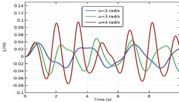
Figure 6. Wave profiles comparison for various values of the amplitude of horizontal excitation, with heterogeneity parameter  $\beta=0.3$ .
