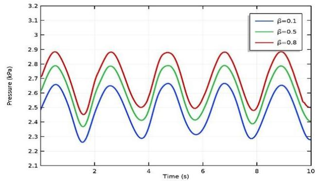
Figure 8. Pressure comparison for various  $\beta$  parameters at position  $(x=L, y=W/2, Z=-0.25\text{ m})$ .
