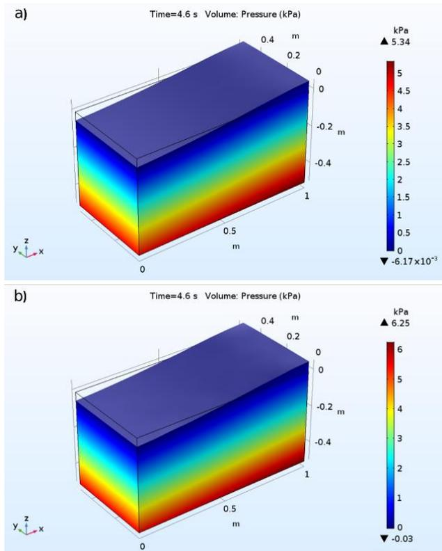
Figure 7. Pressure simulations for various  $\beta$  parameters ( $\beta=0$  for cases a, b and  $\beta=0.5$  for cases c, d), with  $\omega=3\text{ rad/s}$ .
