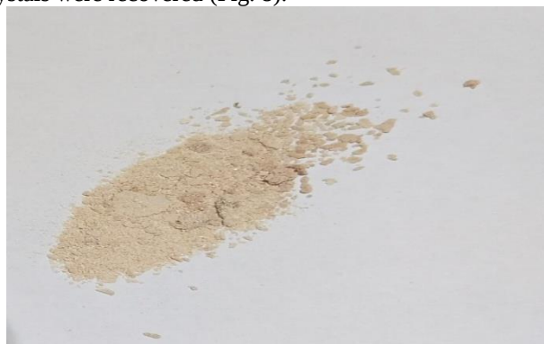
Figure 8: Citric Acid recovered from fermented dehydrated sweet potato peel
