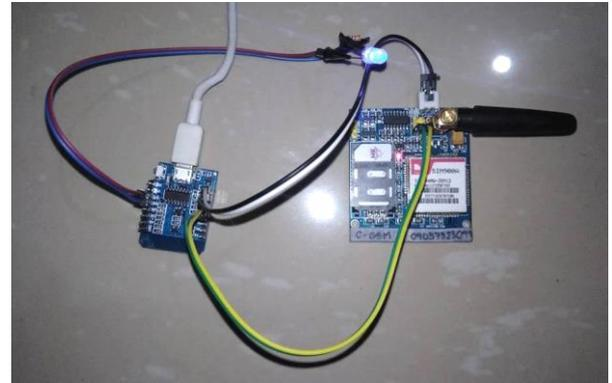
Figure 2. Actual Setup of the SMS Transmitting Device
