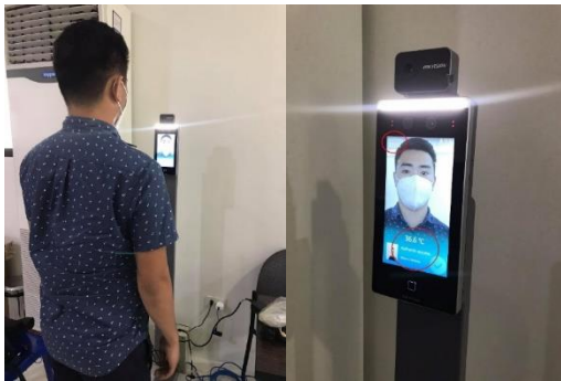
Figure 7. Actual testing of MinMoe device with a USTP Employee's Temperature and Time-Logs sent to HRIS and HIMS
