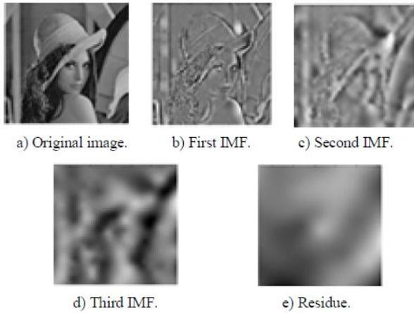
Fig. 1. Example of applying BEMD on Lena image.
