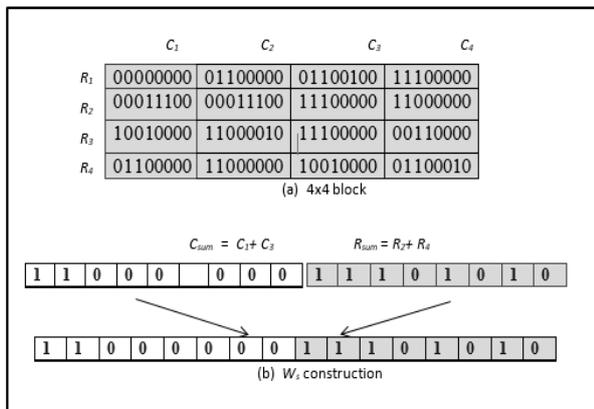
Fig. 4. Example of spatial domain fragile watermark construction
