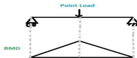
**Figure. 3** Bending Moment diagram due to central point load
