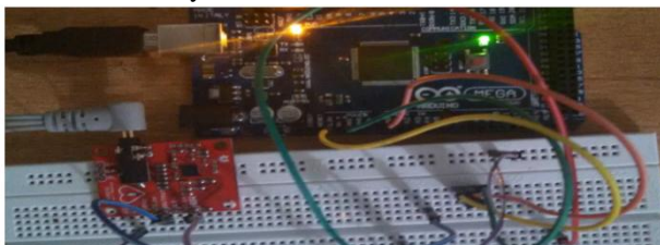
Fig. 5. Arduino-pulse sensor connectivity configuration
