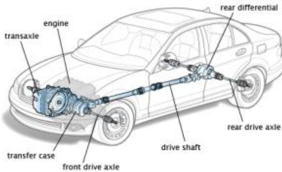
Figure 1 Car driveshaft
