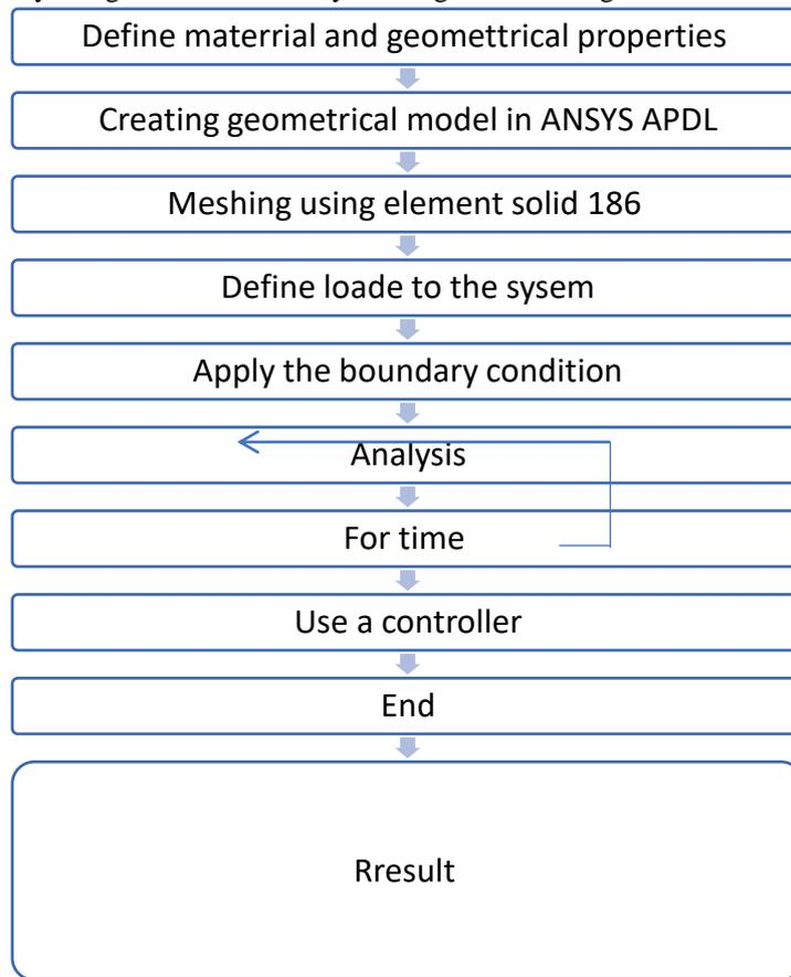
**Figure 3 FGM Flowchart by ANSYS APDL**
