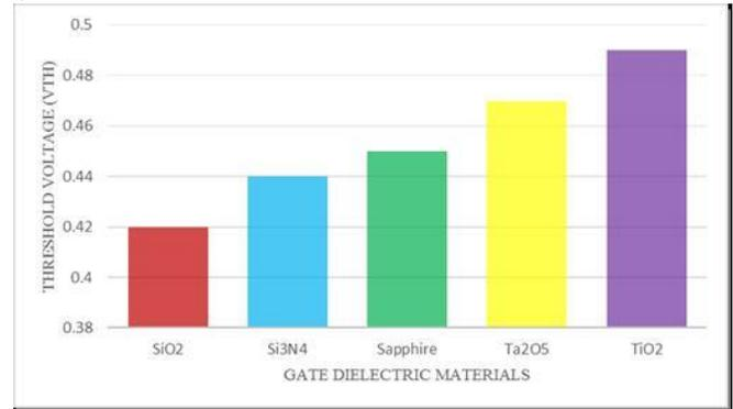
Fig. 2. Threshold Voltage variation for different gate dielectric materials ( $V_d = 0.1V$ )
