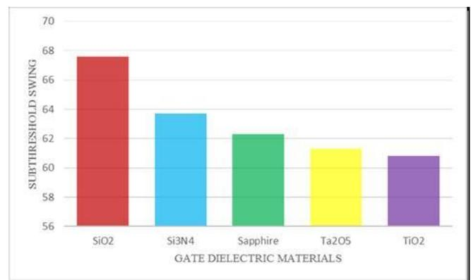
Fig 3. Sub-threshold Swing variation for different gate dielectric materials. ( $V_d = 0.1V$ )
