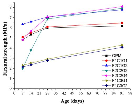
Figure (2) Flexural strength of OPM and specimens with various CFA, CFBCA and GGBFS replacement rates
