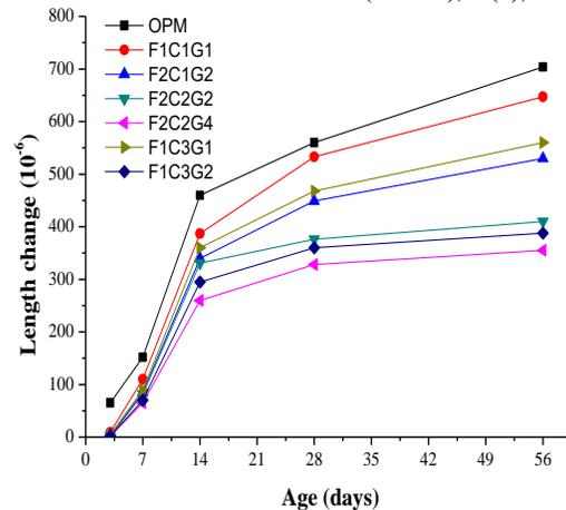
Figure (3) Length change of OPM and specimens with various CFA, CFBCA and GGBFS replacement rates
