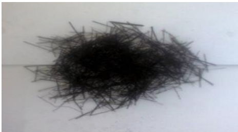
Figure.2 Steel fiber in 1 inch cut length
