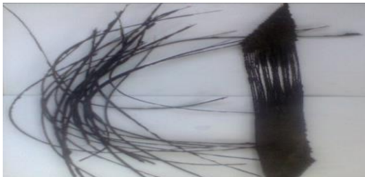
Figure.1 Used tyres steel fibers
