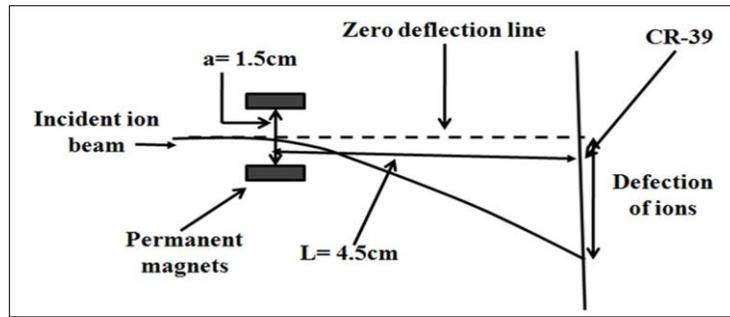
Figure 1: Schematic diagram of Thomson parabola technique.
