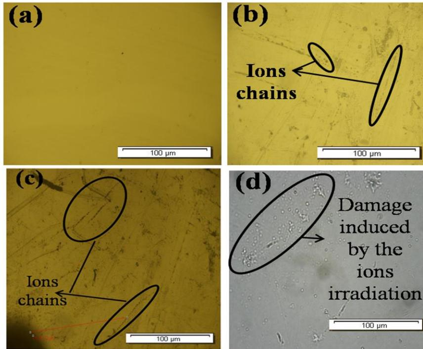
Figure 3: Optical micrographs of (a) pristine PET (b) Al ions, (c) Au ions, (d) Ag ions, irradiated on PET polymer.
