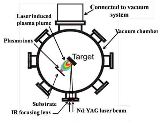
Figure 2: Schematic diagram of ions irradiations setup
