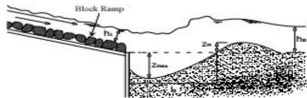
Fig(2) Scour process downstream of a spillway [9]
