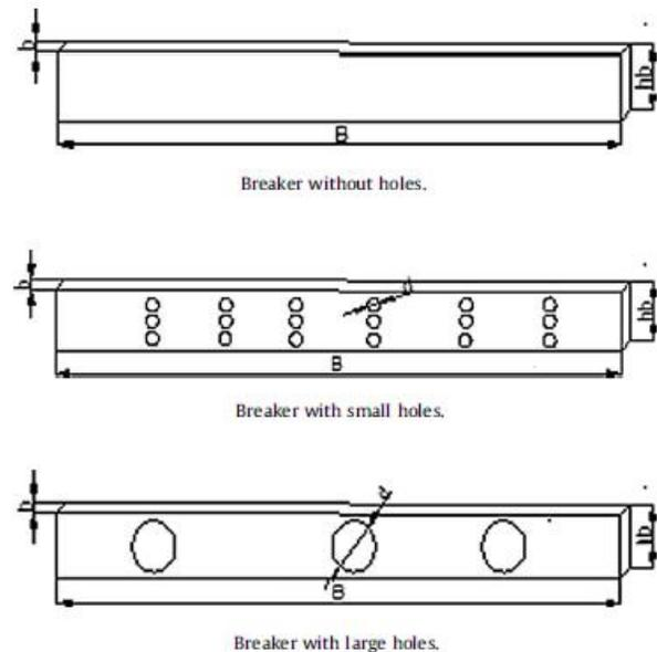
Fig(5) Configuration of breakers [13]
