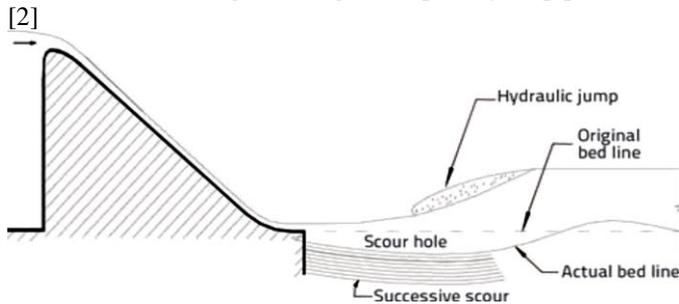
Fig(1) Scour process downstream of a spillway [2]
