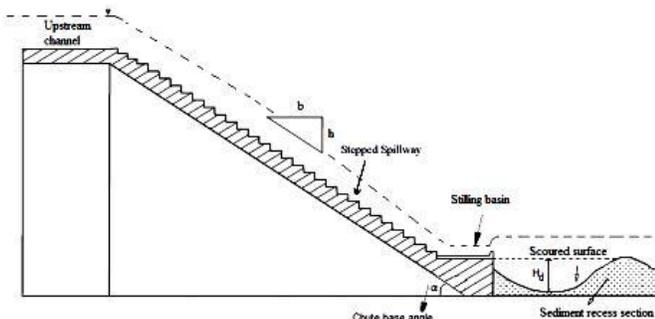
Fig(4) Stepped spillway schematic diagram [10]
