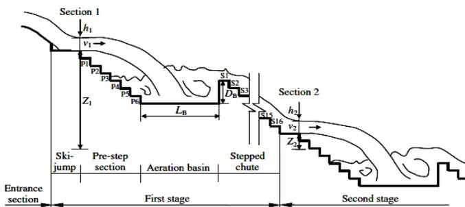
Fig (9) The sketch of ski-jump-step energy dissipator [23]
