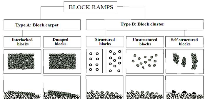
Fig(3) Morphological and structural classification of block ramps [6]
