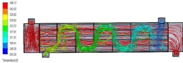
Fig. 3: Temperature cut plots in Heat Exchanger.
