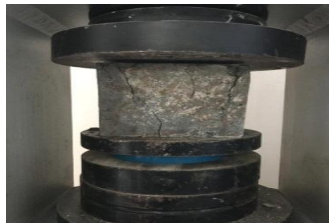
Fig.9 Failure Pattern of Concrete cube
