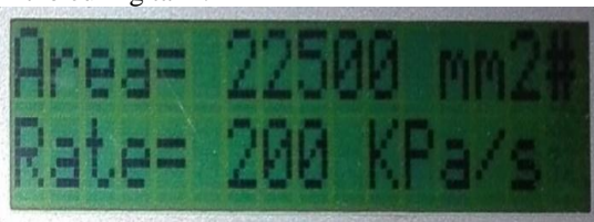
Fig. 3 Setting Area and Load Rate
