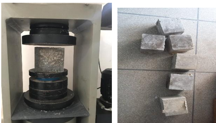
Fig. 4 Compression Testing Machine & Placed Cubes
