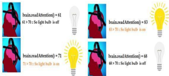
Figure 3. Sample output: Light bulb switched-on if attention value exceeded 70, else remained switched-off.
