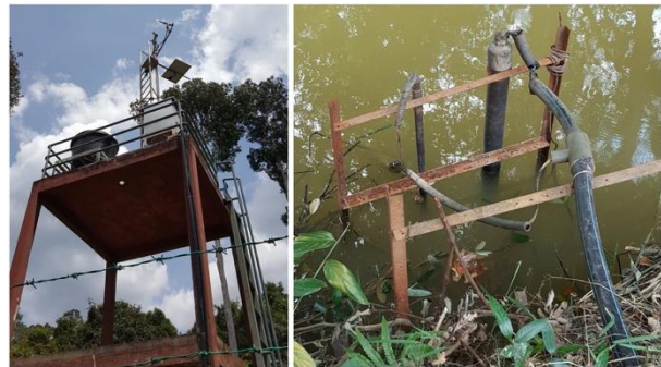
Figure 1. The telemetry tower and water quality sensors.
