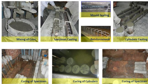
Figure-2 Specimen casting and curing
