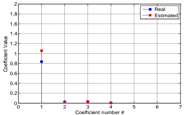
Figure (5): Difference between actual and estimated value of the coefficient of the channel when step size = 0.035
