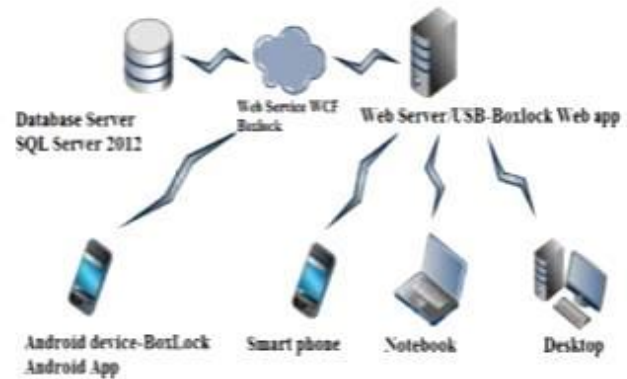
Fig. 4. BoxLock system Architecture
