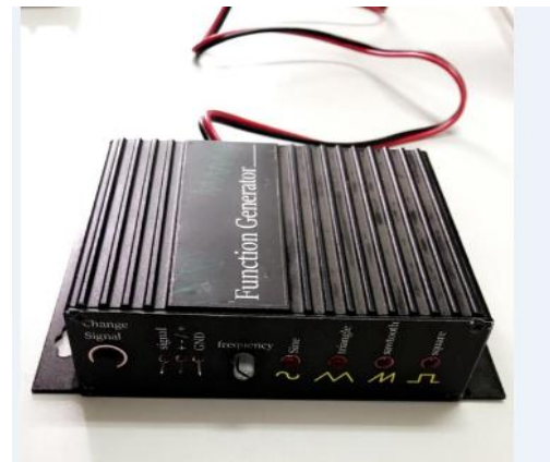
Figure 15: PCB implemented Function generator using lab 11C-207 facilities
