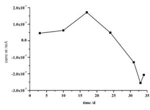
Figure 11. ZRA measurement of copper and iron electrodes [31].
