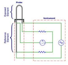
Figure 4. Electrical Resistance Probe [15]
