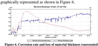
Figure 6. Corrosion rate and loss of material thickness represented against exposure time to corrosive media [18].
