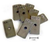
Figure 1. GMW14872 standard mass loss coupons According to GM9540P, the coupons are eligible to be removed after 8 cycles[13].
