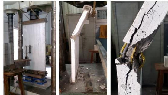
Fig 10: Setup for axial testing of ferro cement panels
