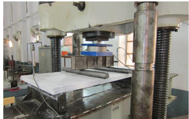
**Fig 4: Setup for flexural testing of ferrocement panels**
