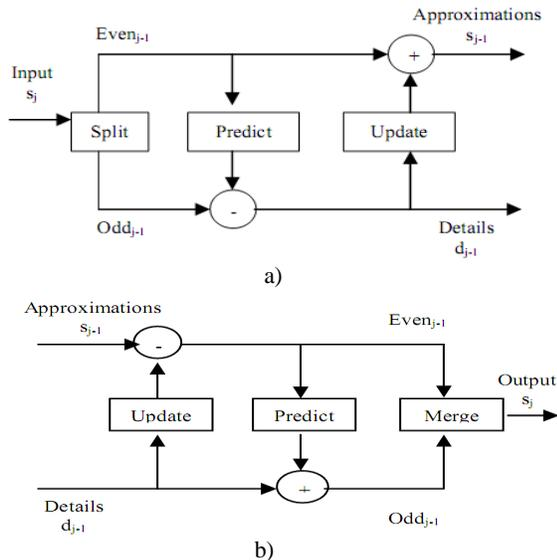
**Fig. 1 Block diagram of lifting transform a) Forward lifting transform and b) Inverse lifting transform**
