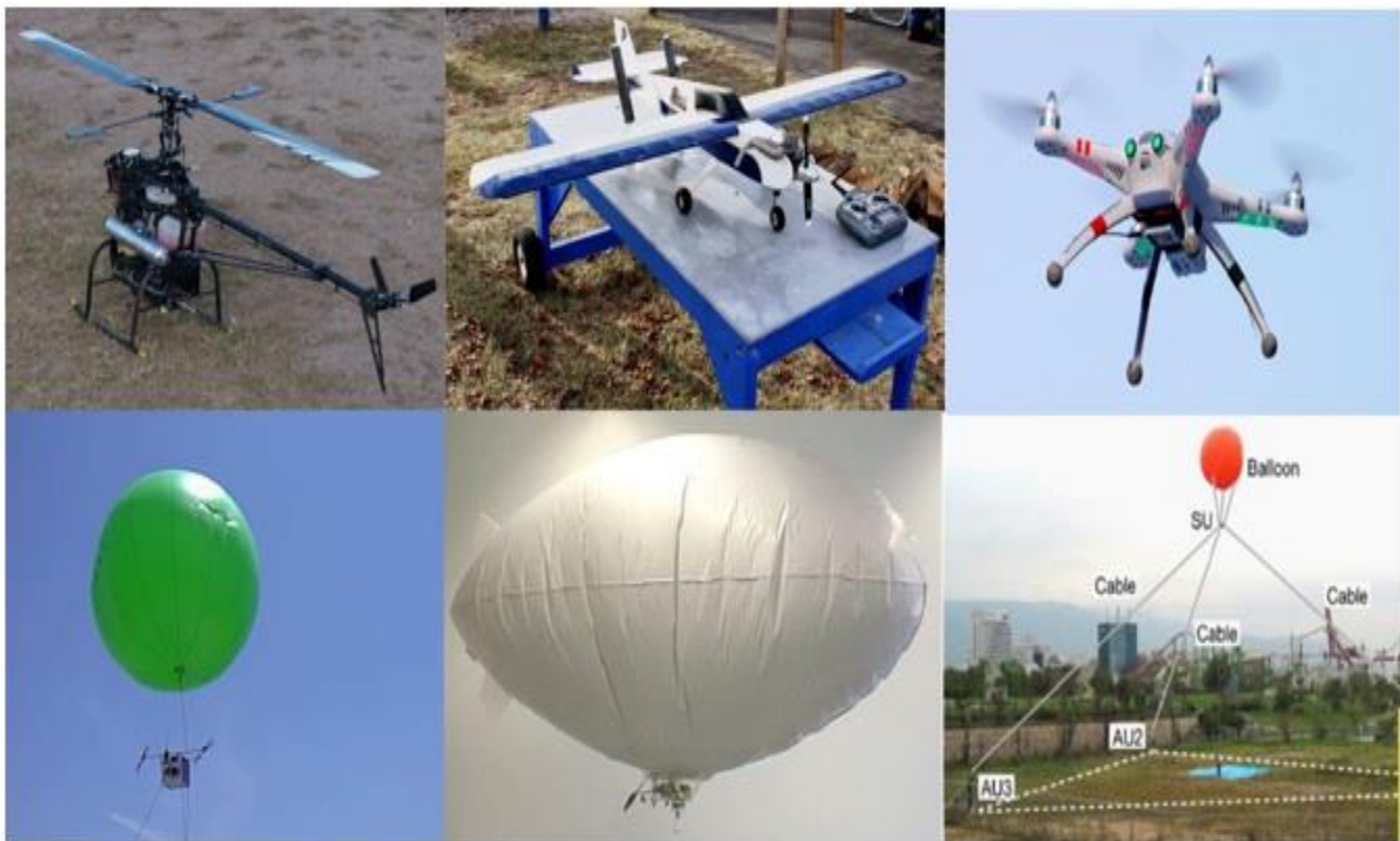
Fig. 2. Different Unmanned Aerial Systems Including, From Left to Right Unmanned Helicopter, Fixed Wing Aircraft, Quad Copter, Balloon Type System, Blimp Type System and Cable Driven Robot. Source:[19]–[23]
