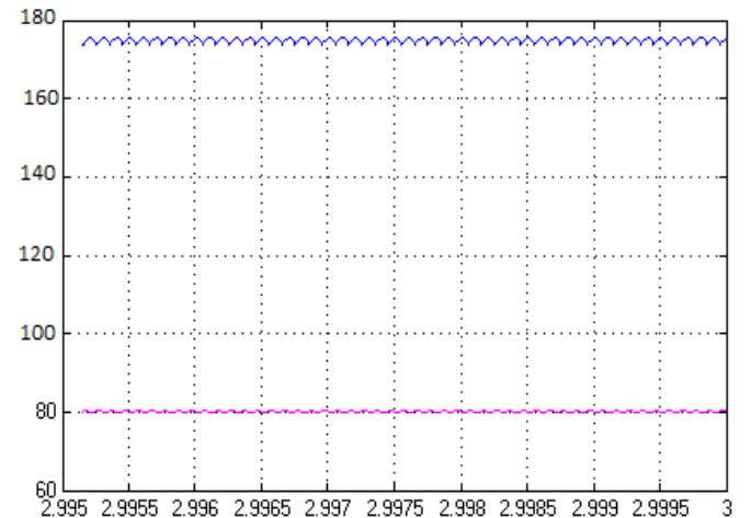
Fig 11: Graph of Boost Converter Voltage and Current
