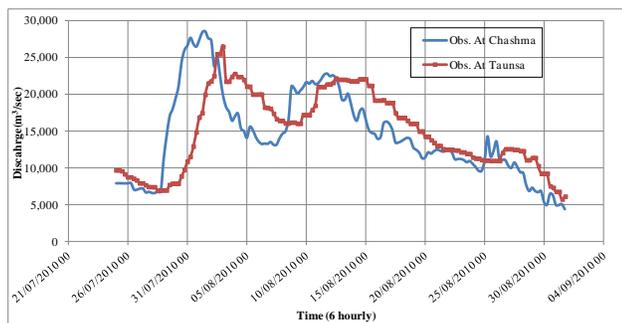
**Figure 1: Observed flow hydrographs at Chashma and Taunsa (2010) (FFC, 2010)**
