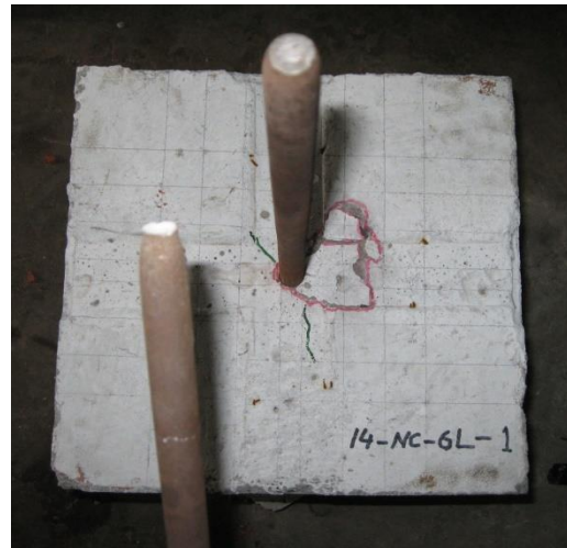
Fig 11: The normal concrete Ø19 L-Anchor of S14 specimen after test. The cracks on top surface and the anchor-bolt steel failure is evident at the rupture load.
