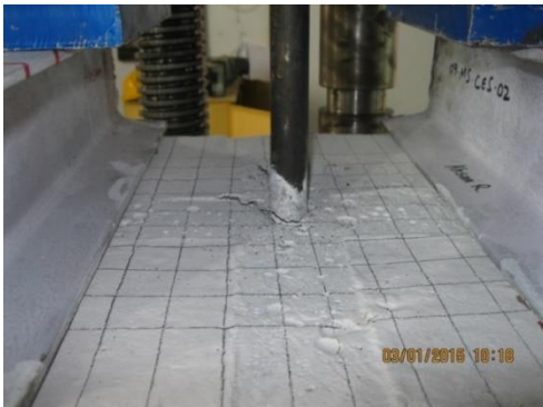
Fig 10: Initial chipping and top surface cracking in surrounding of L-Anchor bolt as the load is entering in-elastic range during testing.
