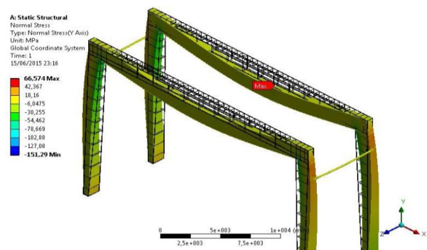
Figure 7a: Normal stress results of simulation for workload of 35 tons
