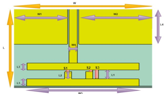
**Fig.1: Triple H-Shaped Patch Antenna**
