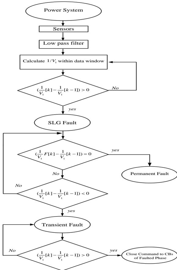
**Figure 7. Flowchart of proposed method for diagnosing fault type and the extinguishing time of secondary arc in PTL**
