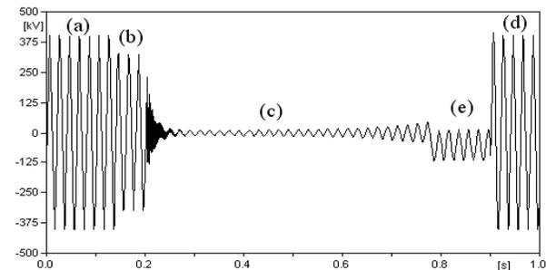
**Figure 3. Voltage waveform of faulted phase at the beginning of line**
