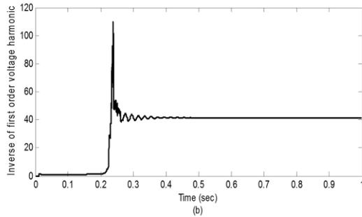
**Figure 6. Voltage waveform of faulted phase at the Sending end of line along with 1/V1 for a permanent fault**
