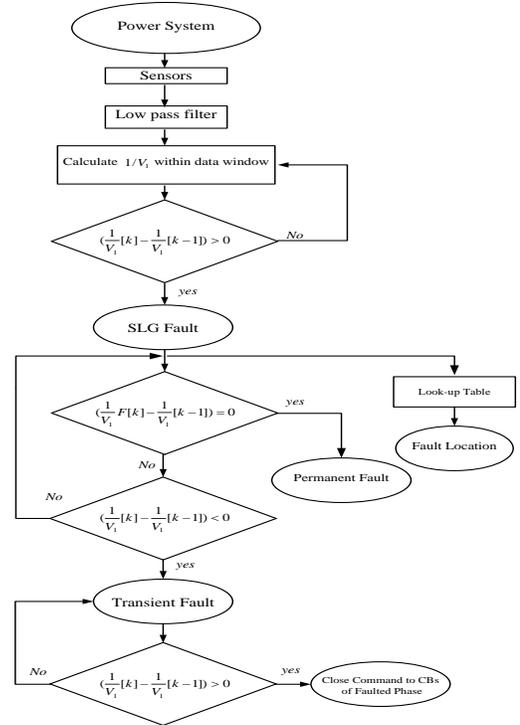
**Figure 10. Flowchart of proposed method for diagnosing fault type, the extinguishing time of secondary arc and fault location in PTL**
