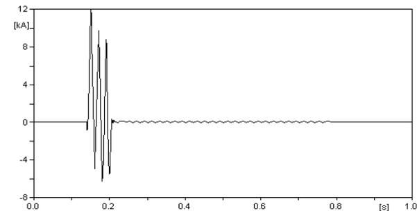
**Figure 4. Current waveform of faulted phase at the beginning of line**
