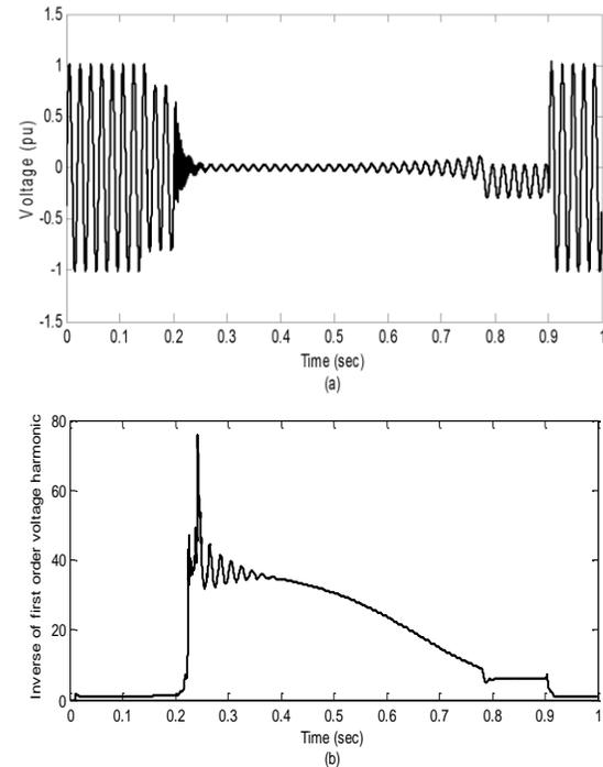
Figure 5. Voltage waveform of faulted phase at the Sending end of line along with  $1/V_1$  for a transient fault
