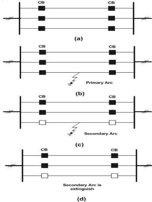
Figure 1. SPAR sequences of operation
