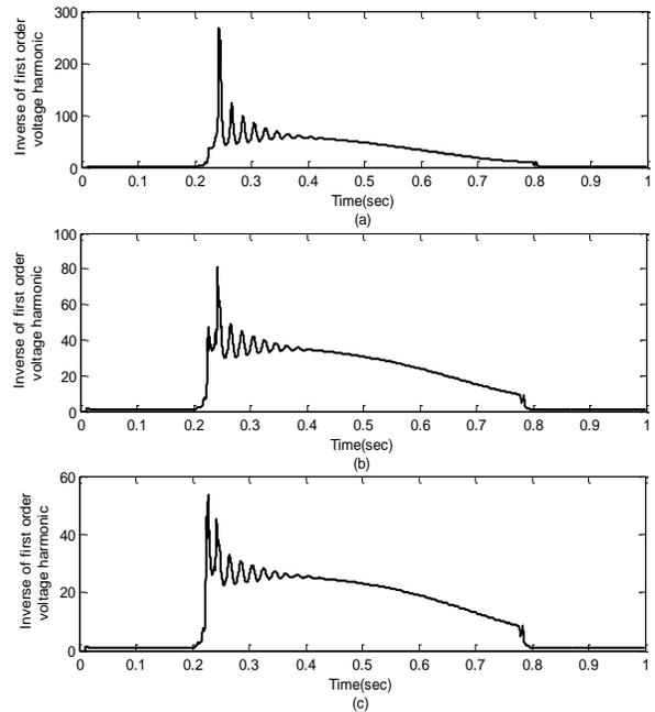
**Figure 8. 1/V1 waveforms of the faulted phase for each of fault locations a) 25% b) 50% and c) 75% far from the voltage measurement location**
