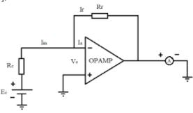
Figure 10. Zero Resistance Ammetry Circuit Diagram [24].
