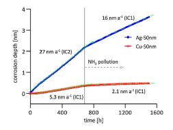
Figure 3. Corrosion depth VS. time for copper and silver[12].
