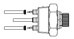
Figure 8. Linear Polarization Resistance Probe[15]
