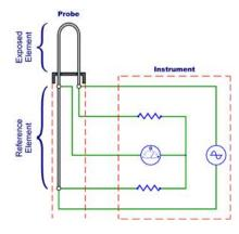
Figure 4. Electrical Resistance Probe [15]
