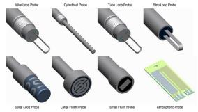
Figure 5. Types of electrical resistance probes[15]
