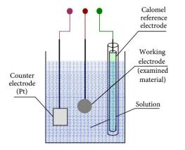
Figure 7. A Sample Three Electrode Cell with Platinum (Pt) Counter Electrode and Calomel Reference Electrode [24].
