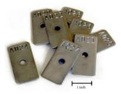
Figure 1. GMW14872 standard mass loss coupons According to GM9540P, the coupons are eligible to be removed after 8 cycles[13].
