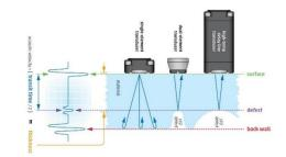
Figure 1 Wall Thickness being measured using ultrasonic transducers [37].
